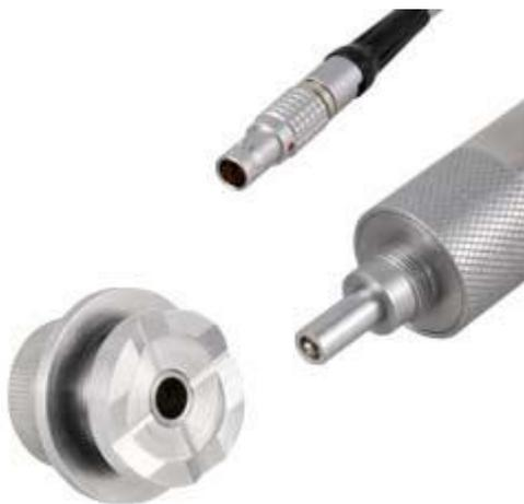
The ultrasonic contact impedance (**UCI**) probe is used for measuring the hardness of small items, objects with a thin wall, complex form, and to measure the hardness of surface hardened layers.
